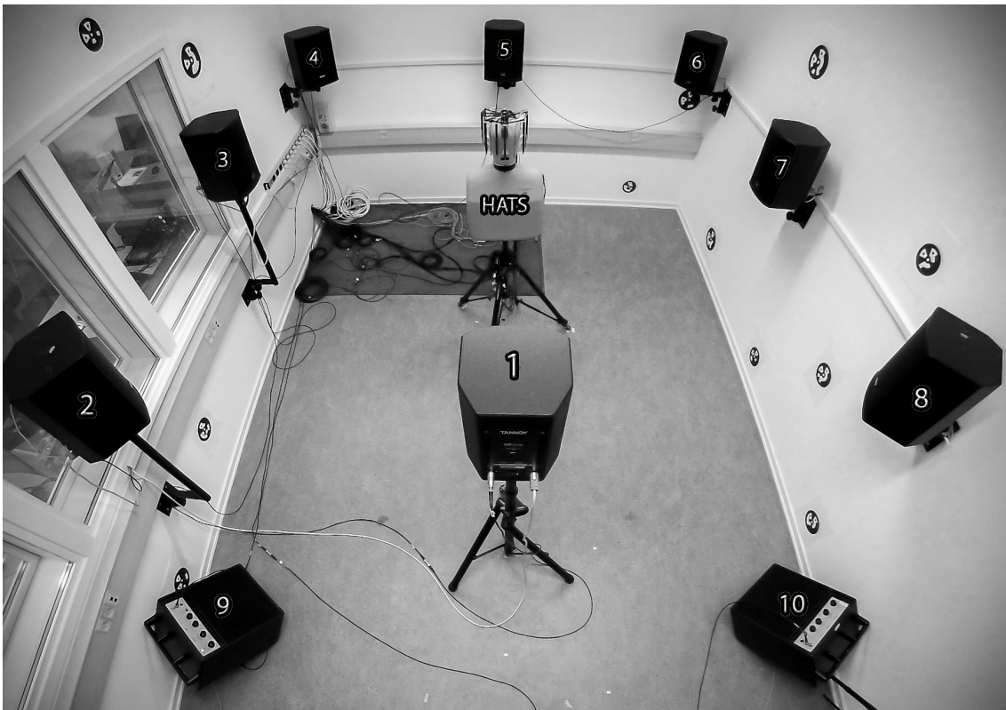
Figure 2.3: Photograph of the loudspeaker array (1 to 8), reference sound sources (9 and 10), and HATS wearing the designed microphone array.
